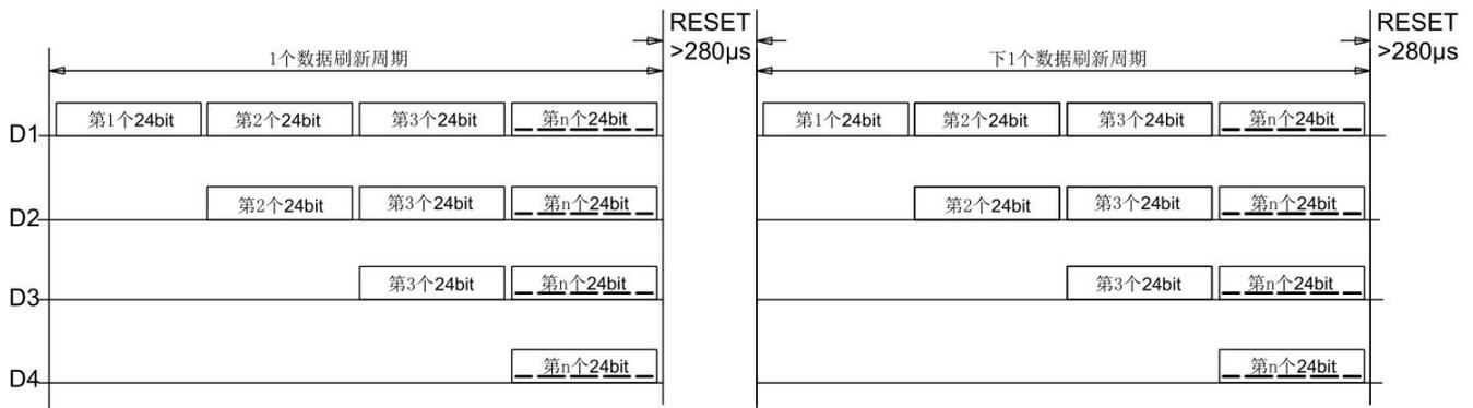
Note: The data of D1 is send by MCU, and D2, D3, D4 through pixel internal reshaping amplification to transmit.
